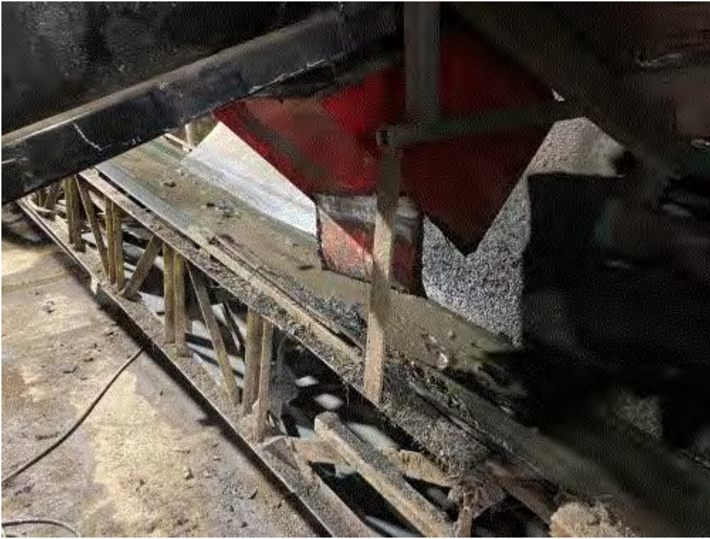
Image 1(1) : Underside of conveyor of 2021-installed tire shredder, showing water and collected particulate.
