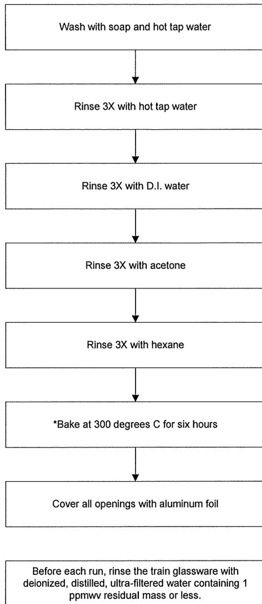
\*As an alternative to baking glassware, a field train proof blank can be performed on the sampling train glassware.
