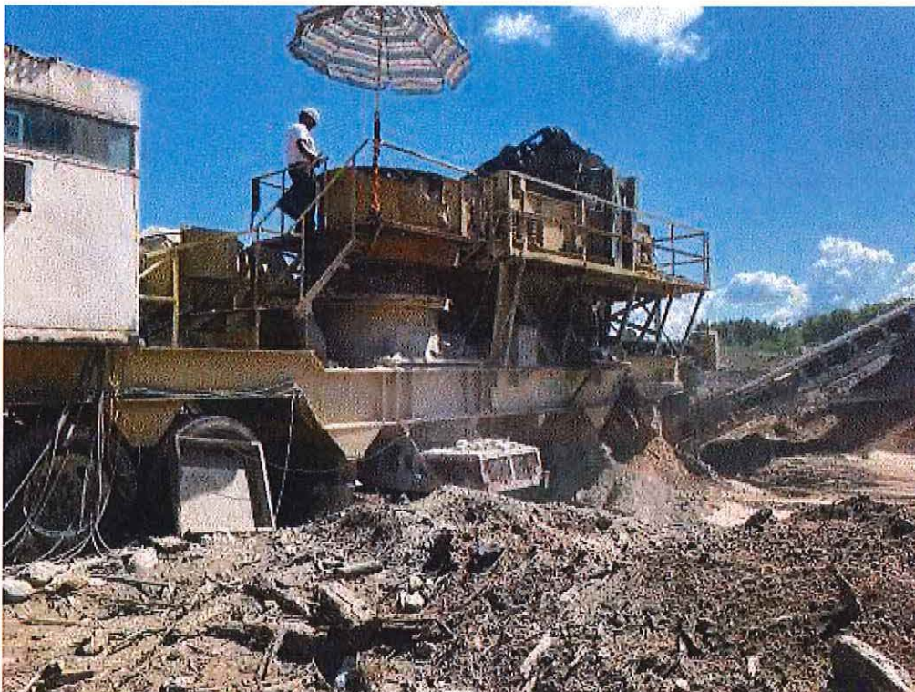
Image 4(Secondary Crusher) : Allis-Chalmers portable crushing plant.
