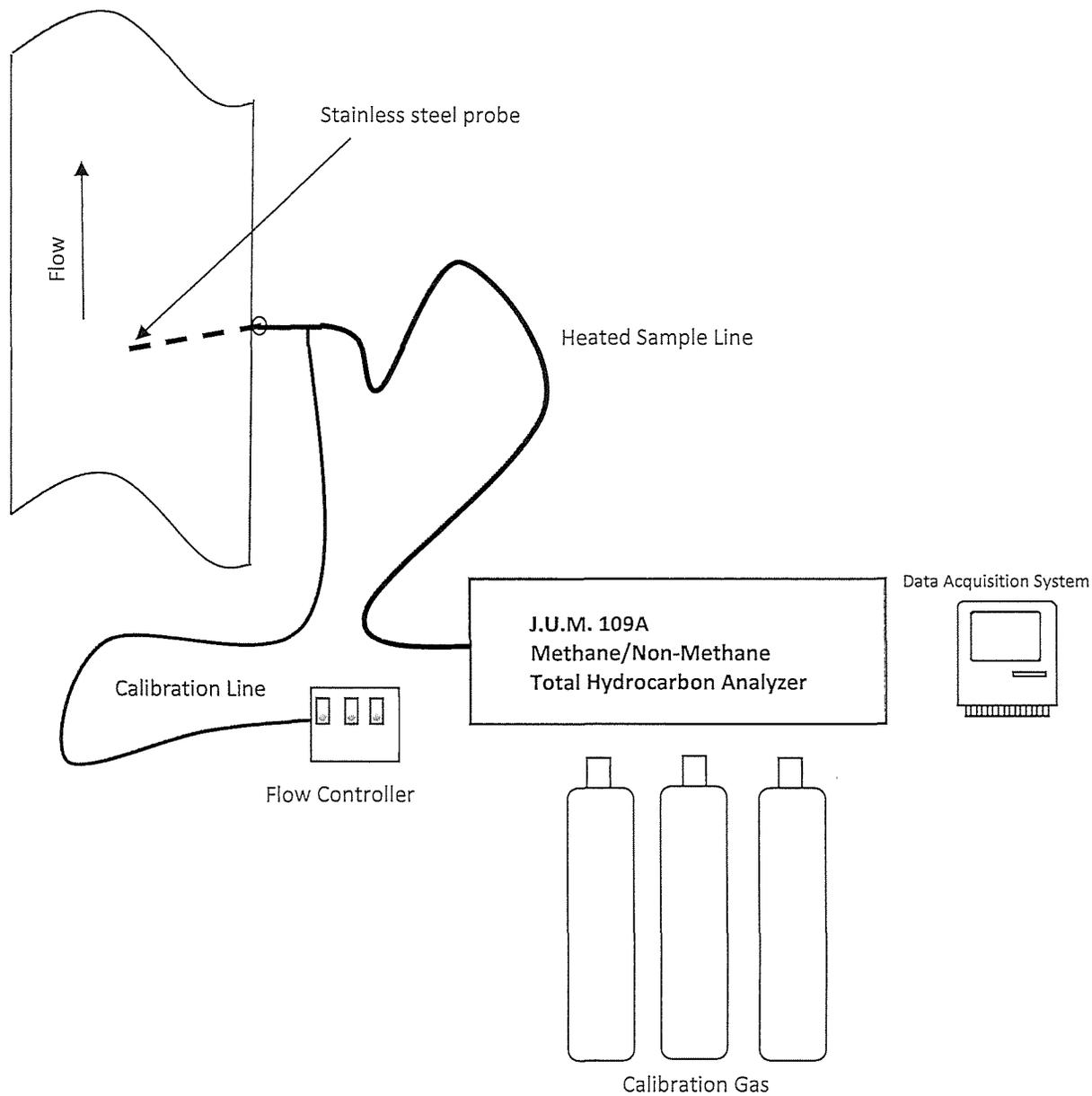
Figure 3 – ASTM D6348/3A
