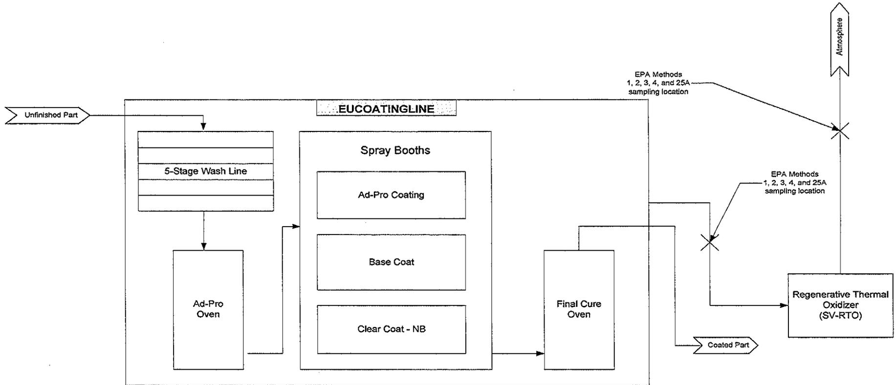
Figure 3.1 - EUCOATINGLINE Process Schematic
