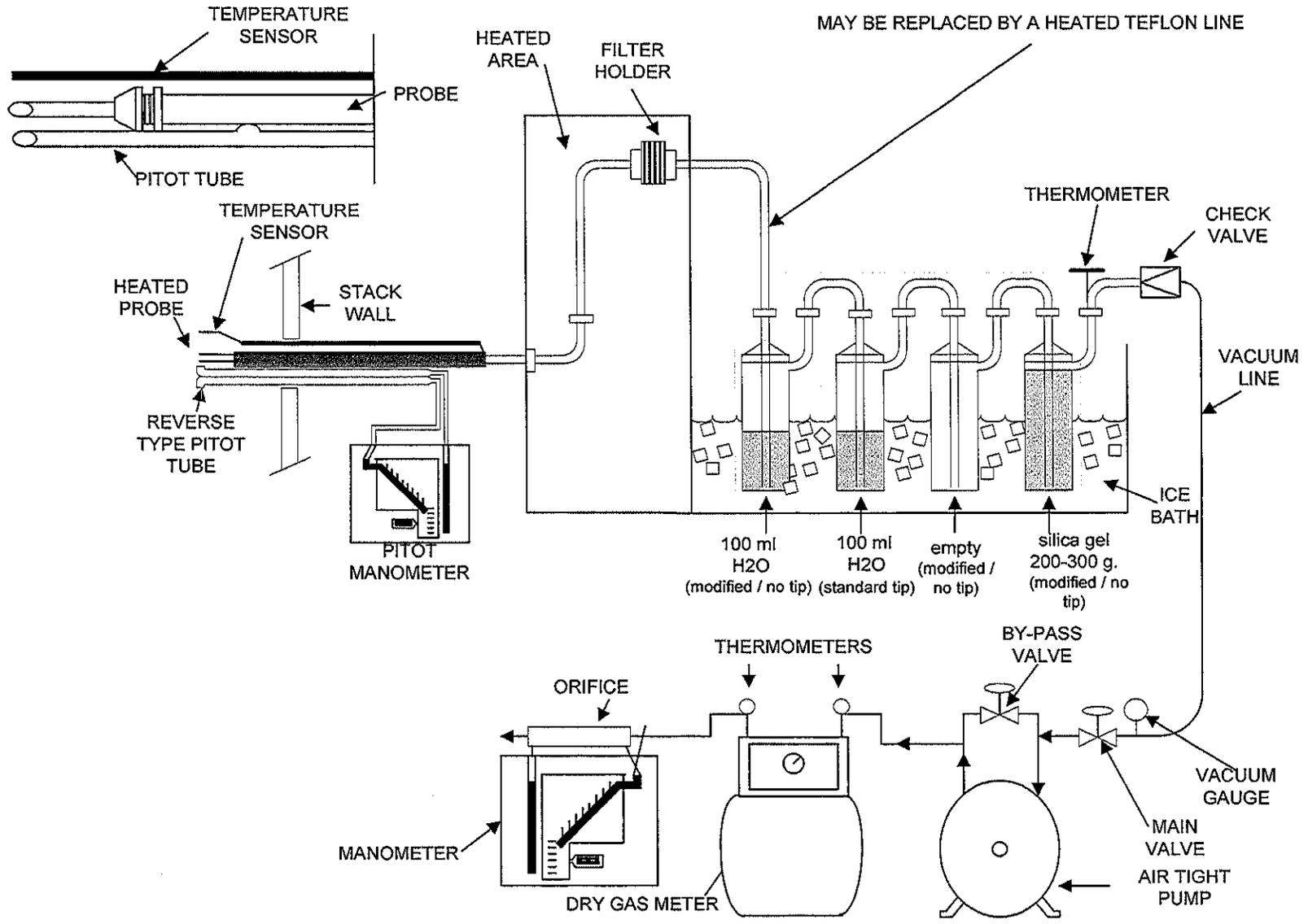
Figure 4.1 - EPA Method 4 Sampling Train Schematic
