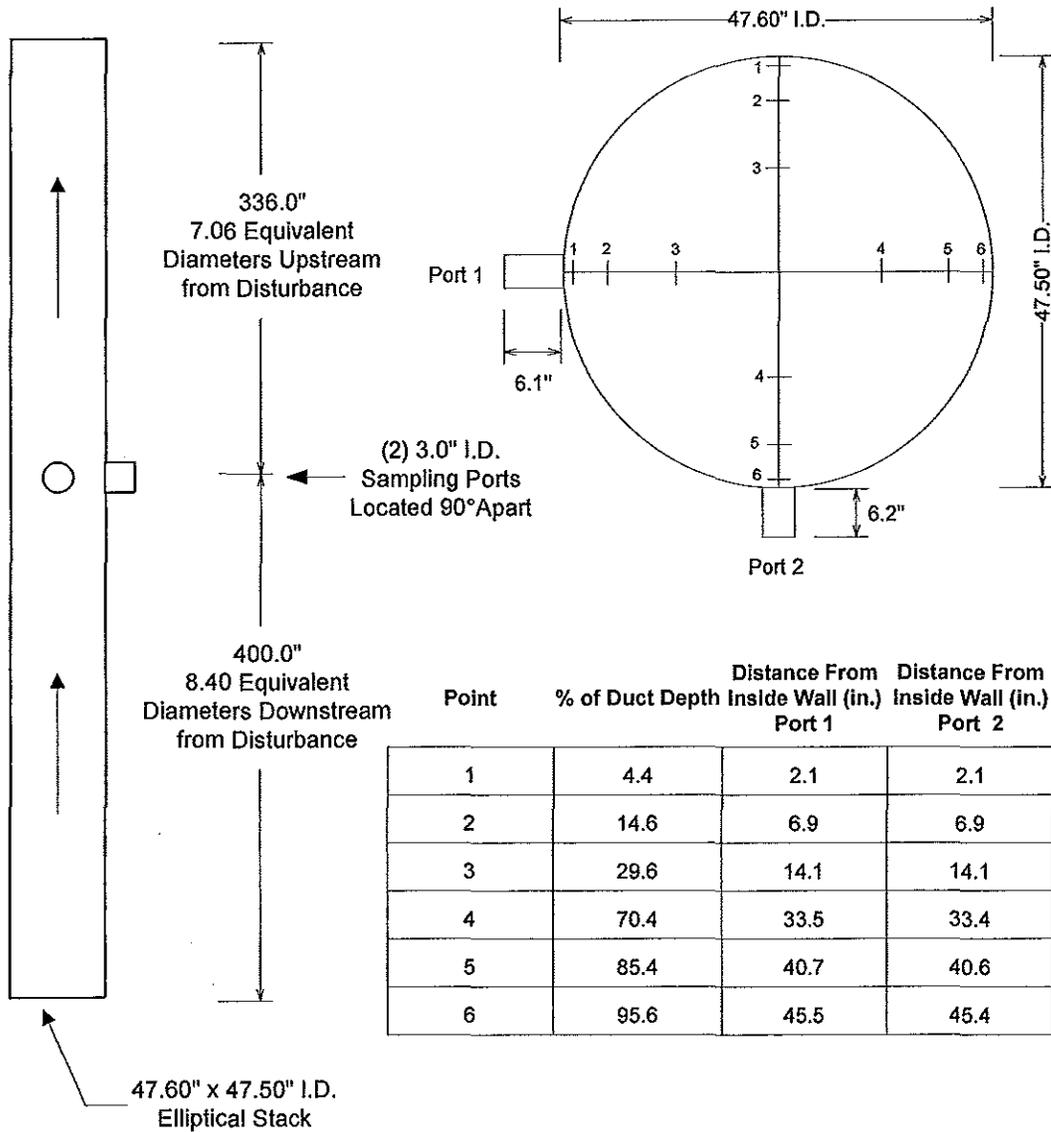
Figure 3.3 - EUCOATINGLINE SV-RTO Exhaust Stack Traverse Point Location Drawing
