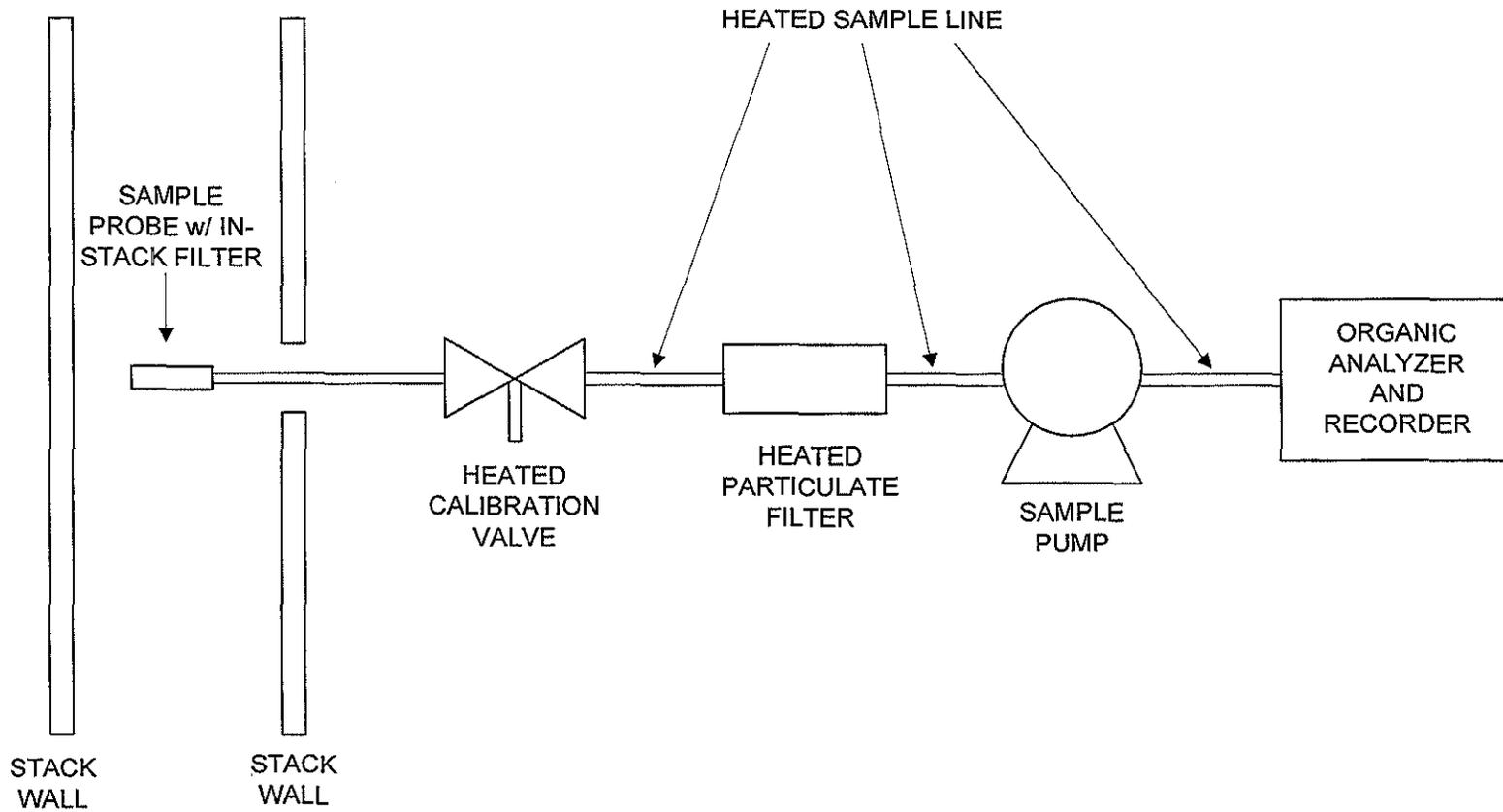
Figure 4.2 - EPA Method 25A Sampling Train Schematic
