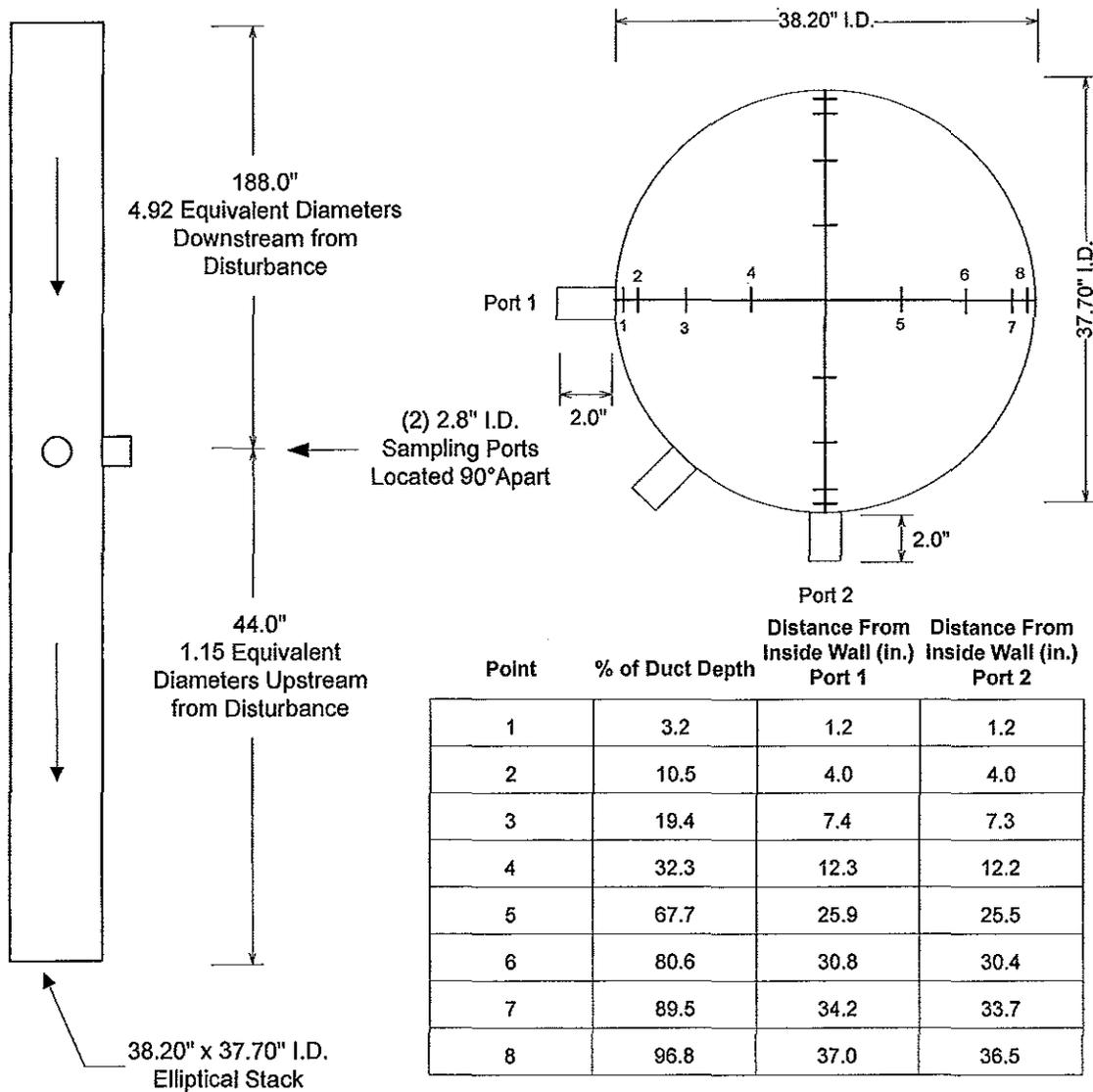
Figure 3.2 - EUCOATINGLINE SV-RTO Inlet Duct Traverse Point Location Drawing
