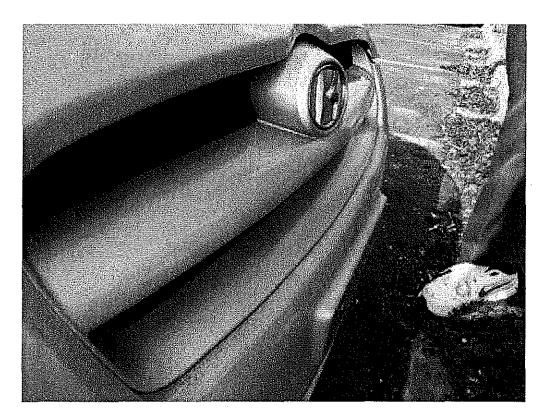
Image 3(Vehicle): Rust like material built up on plastic.
