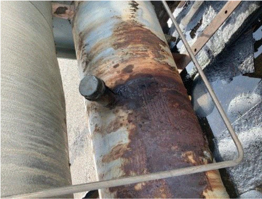
Image 8(Dehy - Small Leak) : Shows the tank that is leaking, absorbent pads, and the leak being captured by secondary containment.
