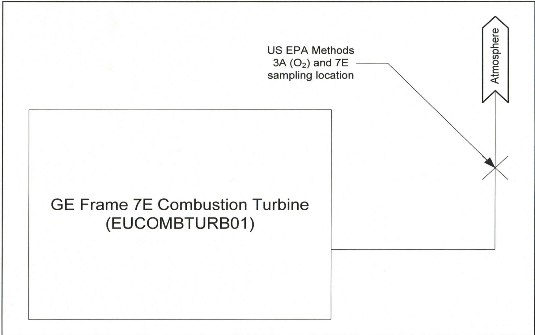
**EUCOMBTURB01 EXHAUST STACK TRAVERSE POINT LOCATION DRAWING**
