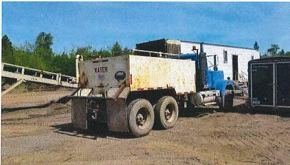
**Image 3(AL3)** : Water truck providing adequate water--no issues with spray bars or fugitive dust.
