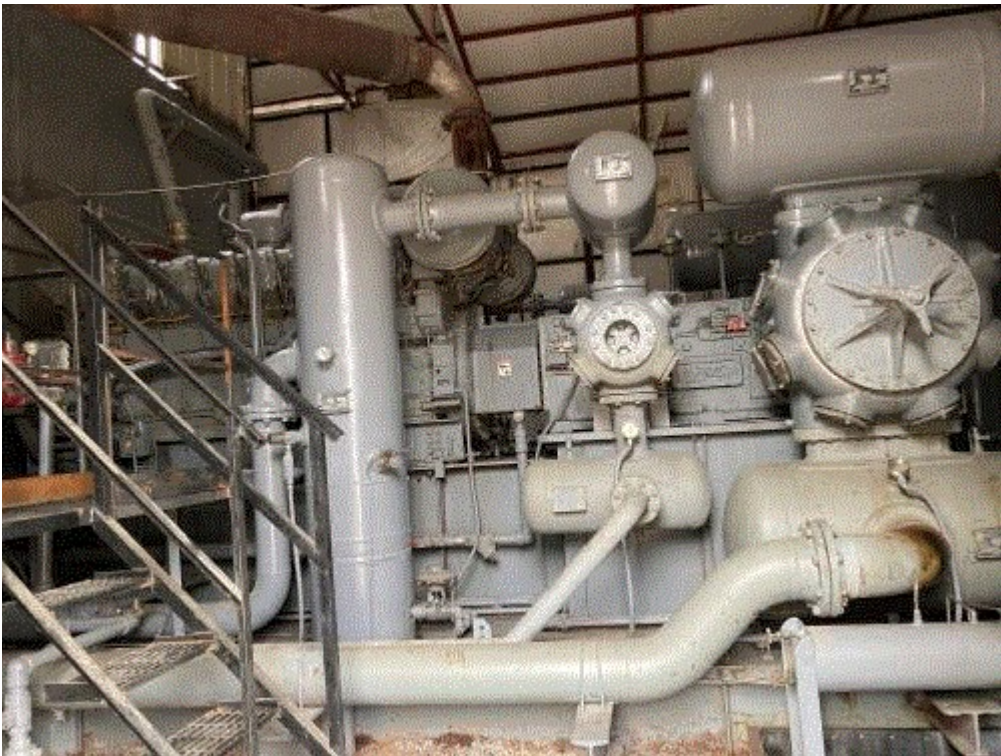
Image 3(CAT3516TA) : 16 Cylinder Engine, 1400 RPM, 1,266 HP
