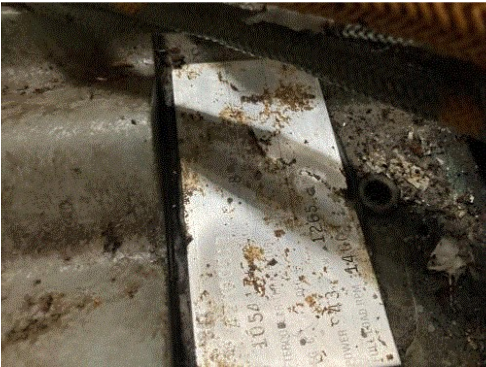
Image 5(Engine Tag) : Serial # 4ZK00612, 1265 HP and 1400 RPM Engine
