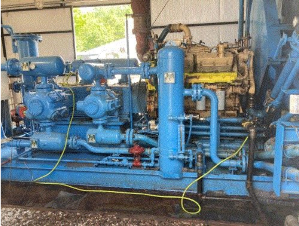
Image 1(Caterpillar Engine) : G3412CLE is a Caterpillar V-12, 4-stroke engine that is rated at 637 HP and operates without a catalytic converter. It was installed November 5, 2020. Skid # CC1199.
