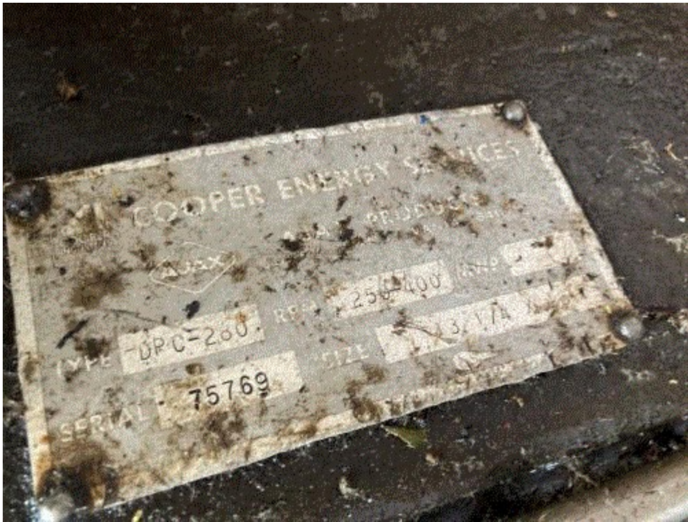
Image 2(Name Plate) : Ajax Name Plate found on Engine.
