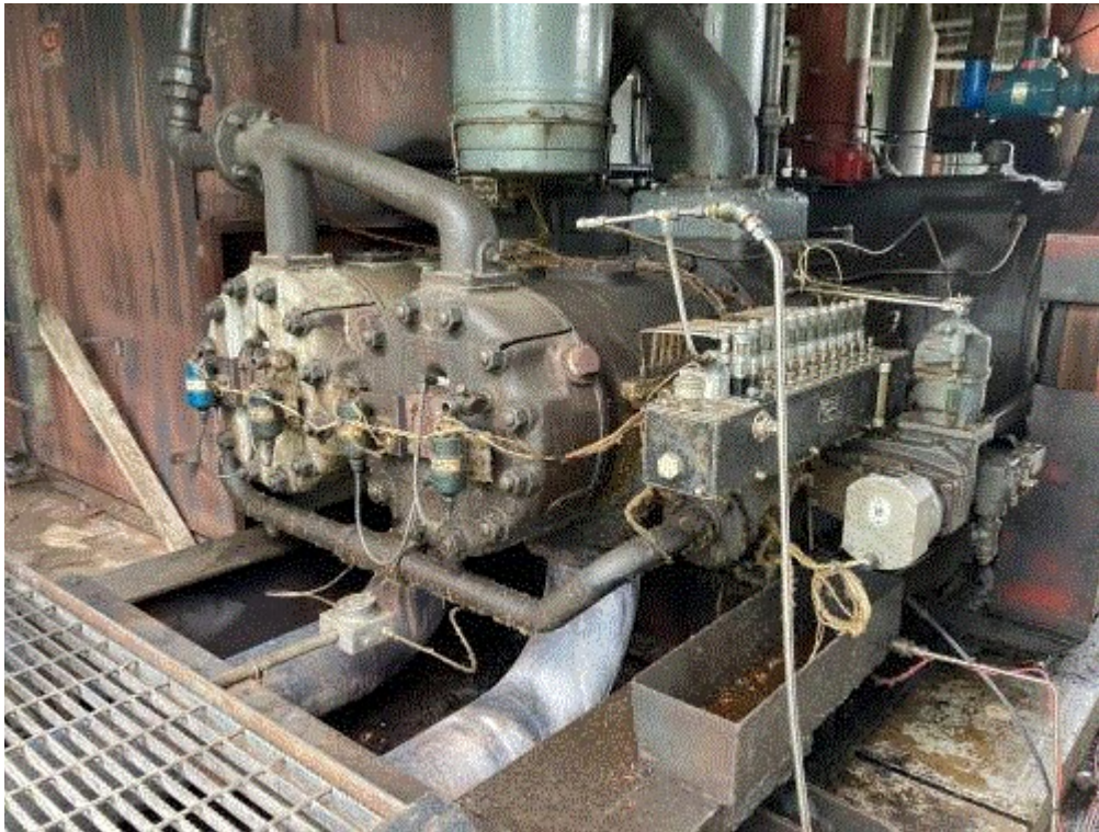
Image 1(AJAX Engine) : EUENGINE1 - Ajax Compressor Engine, Type DPC-280; serial number 75769. Is a 269 HP Engine.
