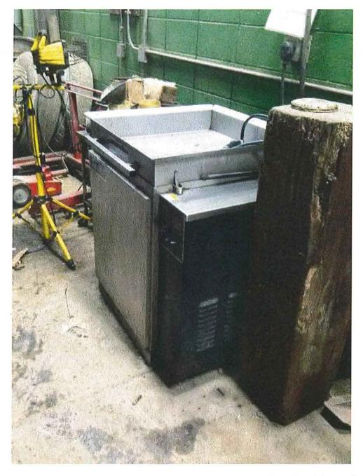
Image 1(ME1): Safety Kleen parts washer using aqueous-based solvent which replaced the small parts washer utilizing halogenated solvents.
