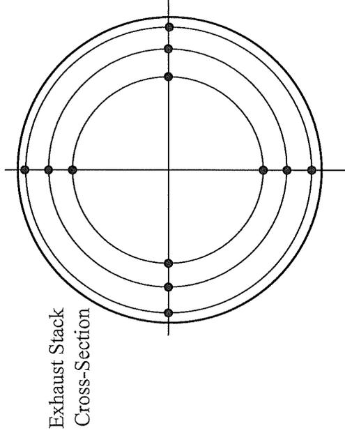
Velocity sample locations as measured from stack wall
