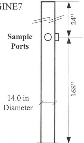
Exhaust Stack Cross-Section
