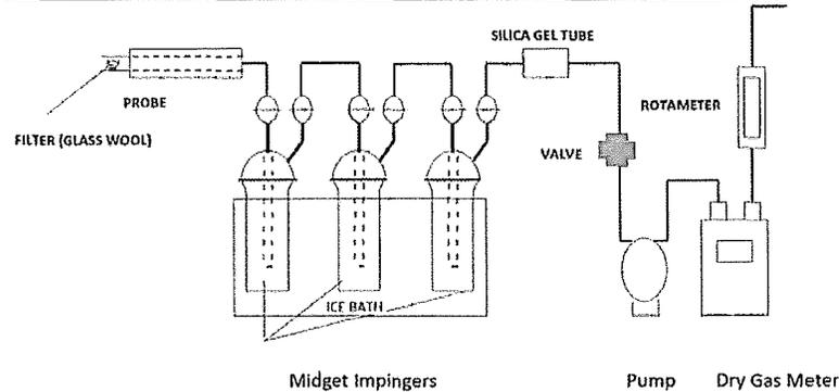
The silica gel tube depicted in this figure was replaced with a midget impinger (bubbler) with a straight tube insert, as allowed in ALT-008, §1
