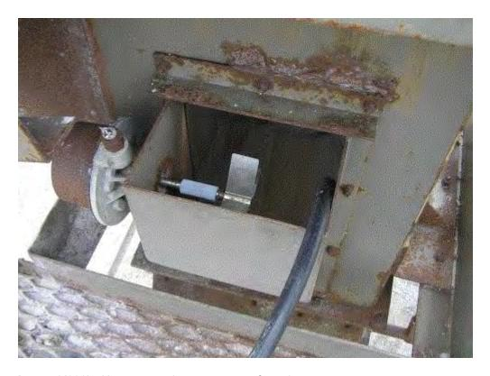
Image 2(002): Hose to supply water to transfer point.
