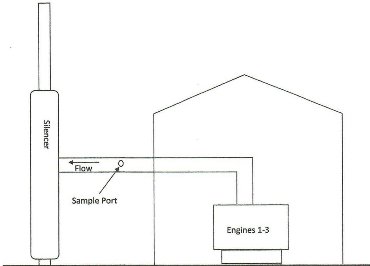
Figure 2 – USEPA Method 3A & ASTM D6348
