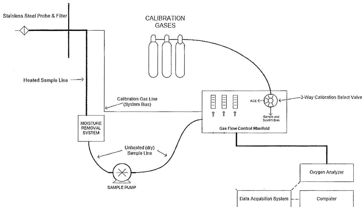
Upon successful completion of the ACE and initial system bias tests, sample flow rates and component temperatures are verified, and the probe is inserted into the stack. After confirming the unit is operating at established conditions, the sampling commences. Gas concentrations were recorded at 1-minute intervals throughout the test program.
