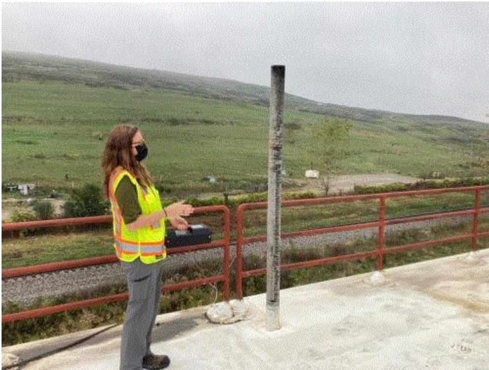
**Image 2(Passive vent)** : Passive vent from condensate sump. Measured methane at 129,000 ppm with measured H<sub>2</sub>S greater than 50 ppm.
