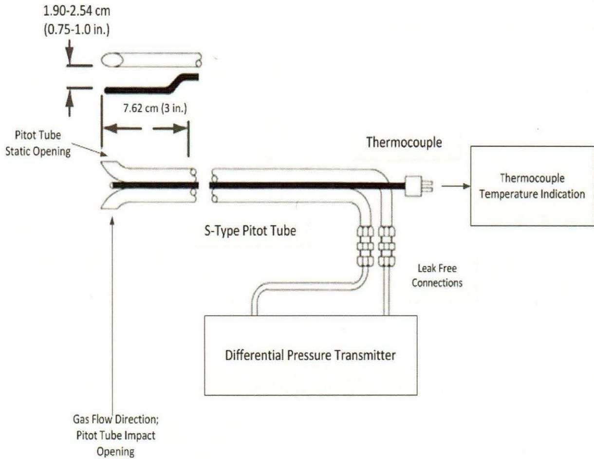
Figure 4 – ALT-008 Moisture Sample Apparatus
