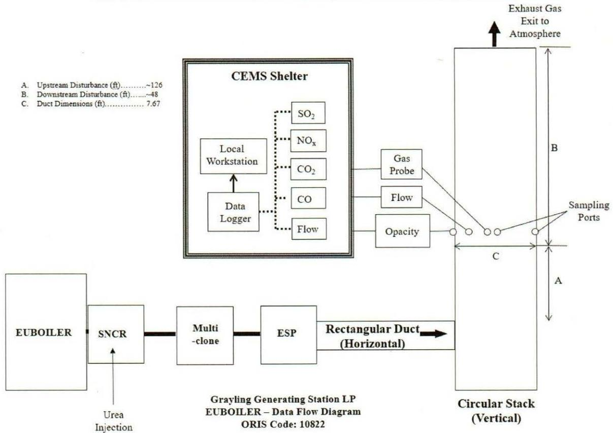
Figure 2 – EUBOILER Flow Traverse Points Dimensions and Detail
