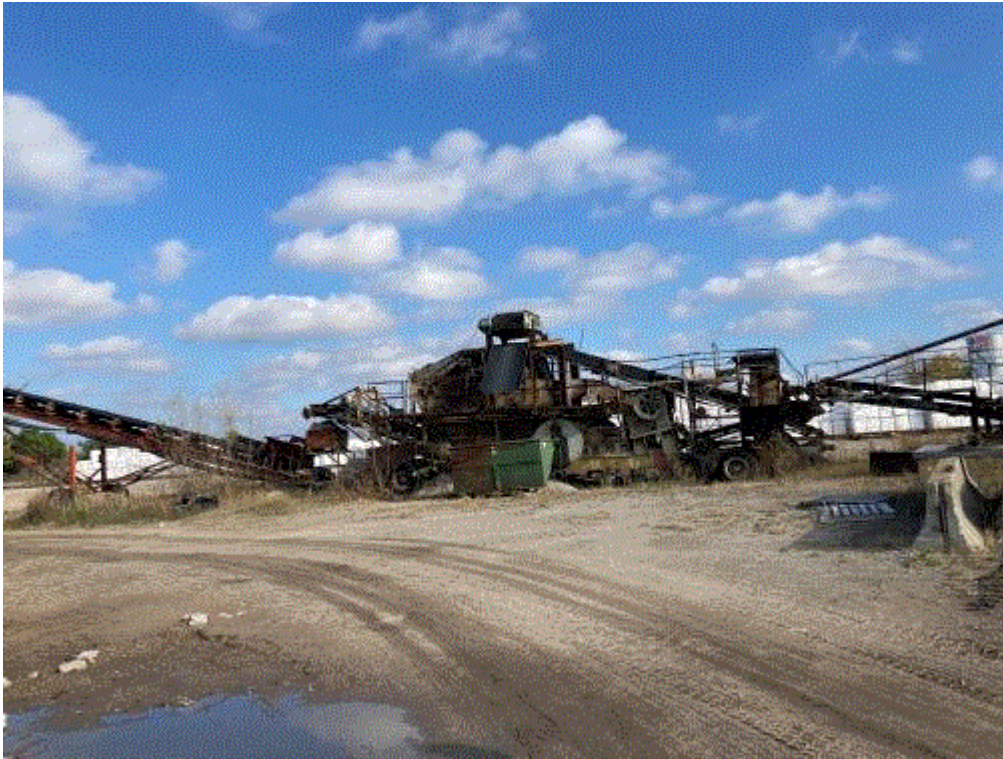
Image 3(Crushing Unit 1) : The Rusted Crusher that is hooked up to the generator, multiple conveyors and located near the well for dust suppression.
