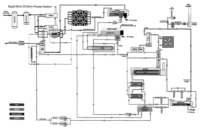
Figure 2-2. Rapid River 35 Dehydration Unit Process Flow
