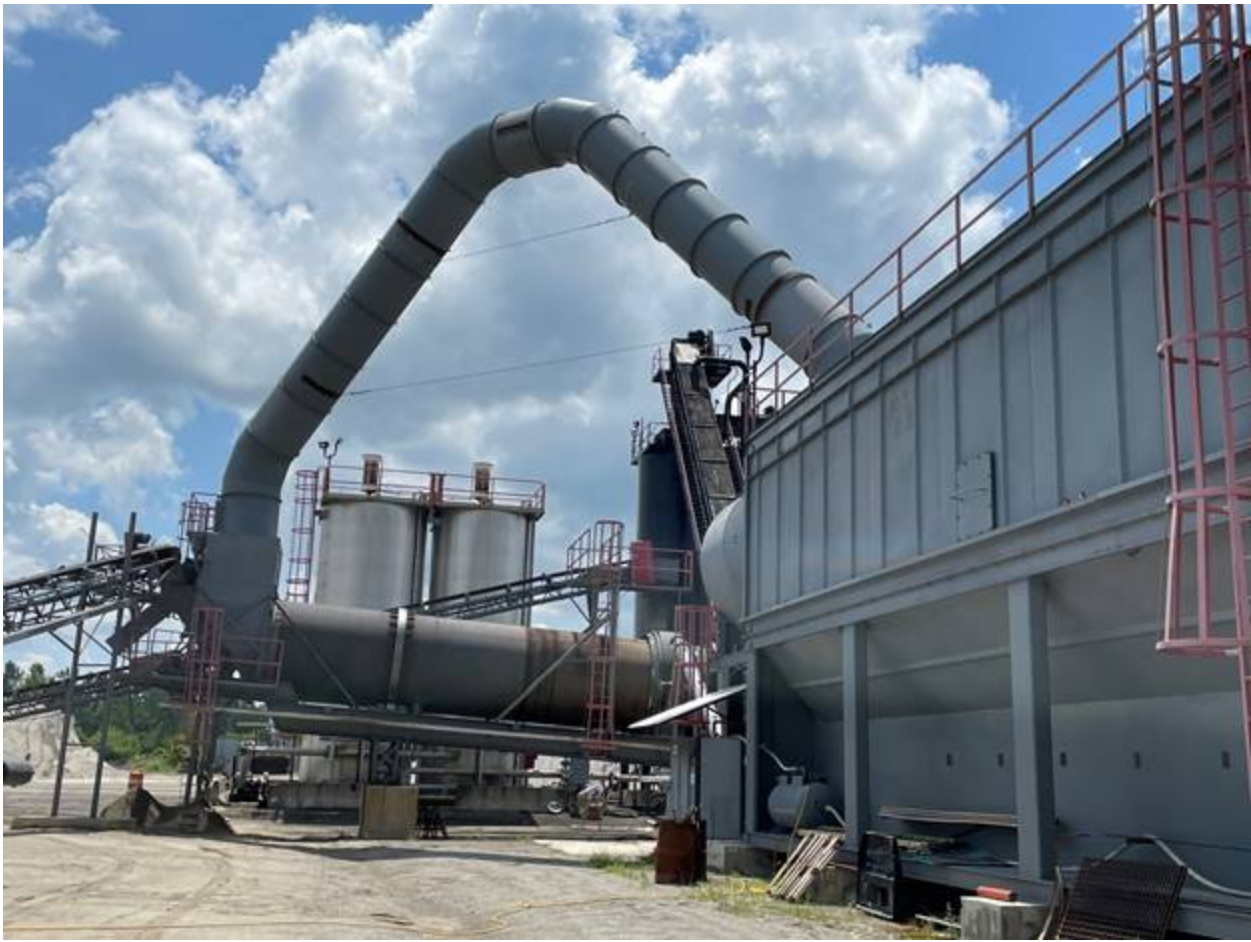
Image 7: Rotary drum. Aggregate is fed from the left, and exits the drum to the right and is conveyed up into the storage tanks.
