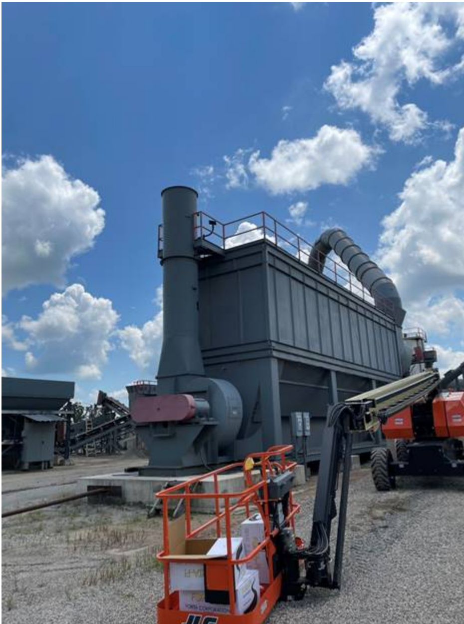
Image 6: Baghouse with aggregate hoppers to the back left.
