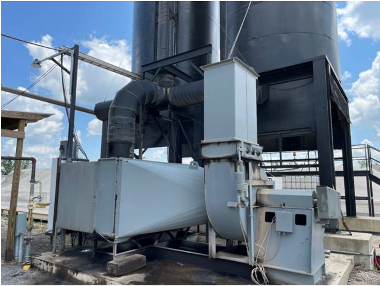
Image 5: Blue Smoke collection system with storage tanks.
