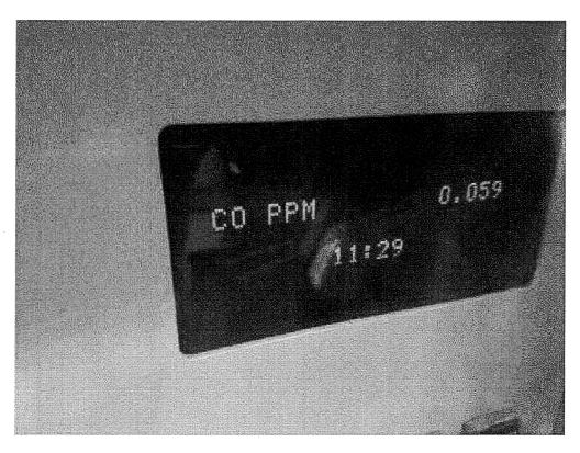
Image 15(CEMS Control Room) : CO reading of 0.059 ppm
