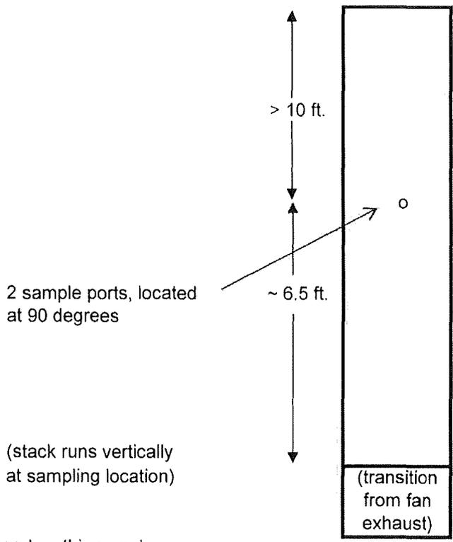
Stack Diameter: 36 inch (stack runs vertically at sampling location)
