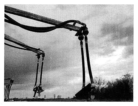
Image 1(Loading arms): Loading arms which show break-away shutoff device.
