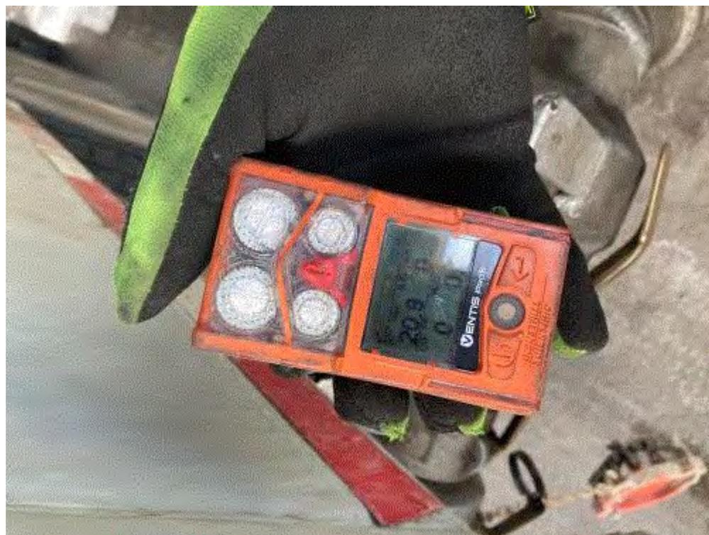
**Image 4(LEL Meter) :** Meter used to check for leaks. Reading was "0" during inspection.
