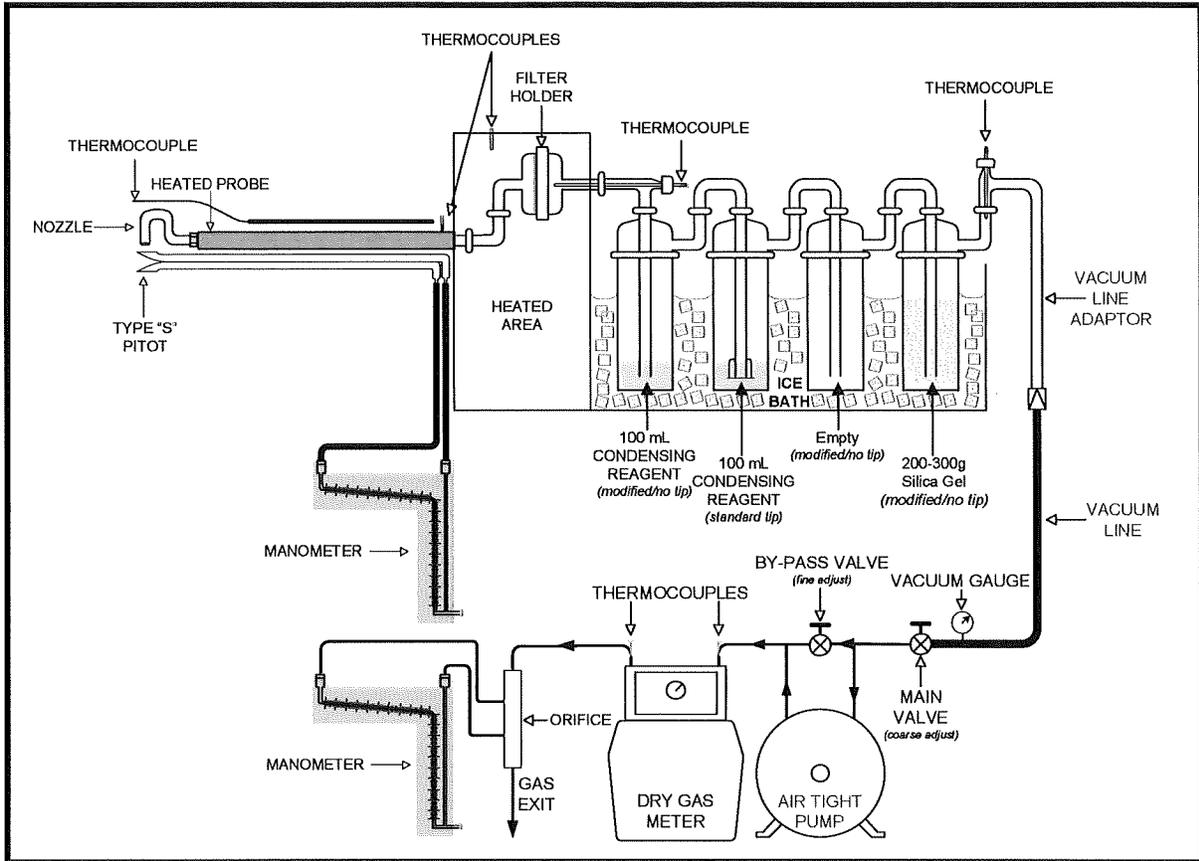
**3.1.6 EPA Method 19, Determination of Sulfur Dioxide Removal Efficiency and Particulate Matter, Sulfur Dioxide, and Nitrogen Oxide Emission Rates**
