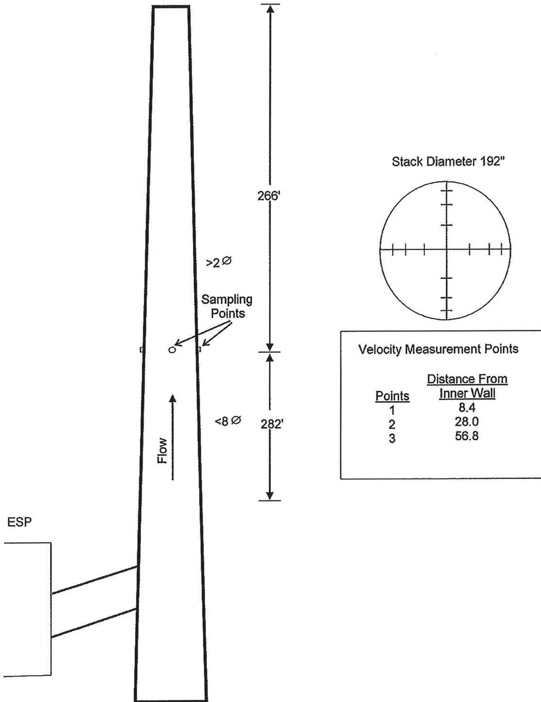
Figure 2 – USEPA Method 26A (Modified)
