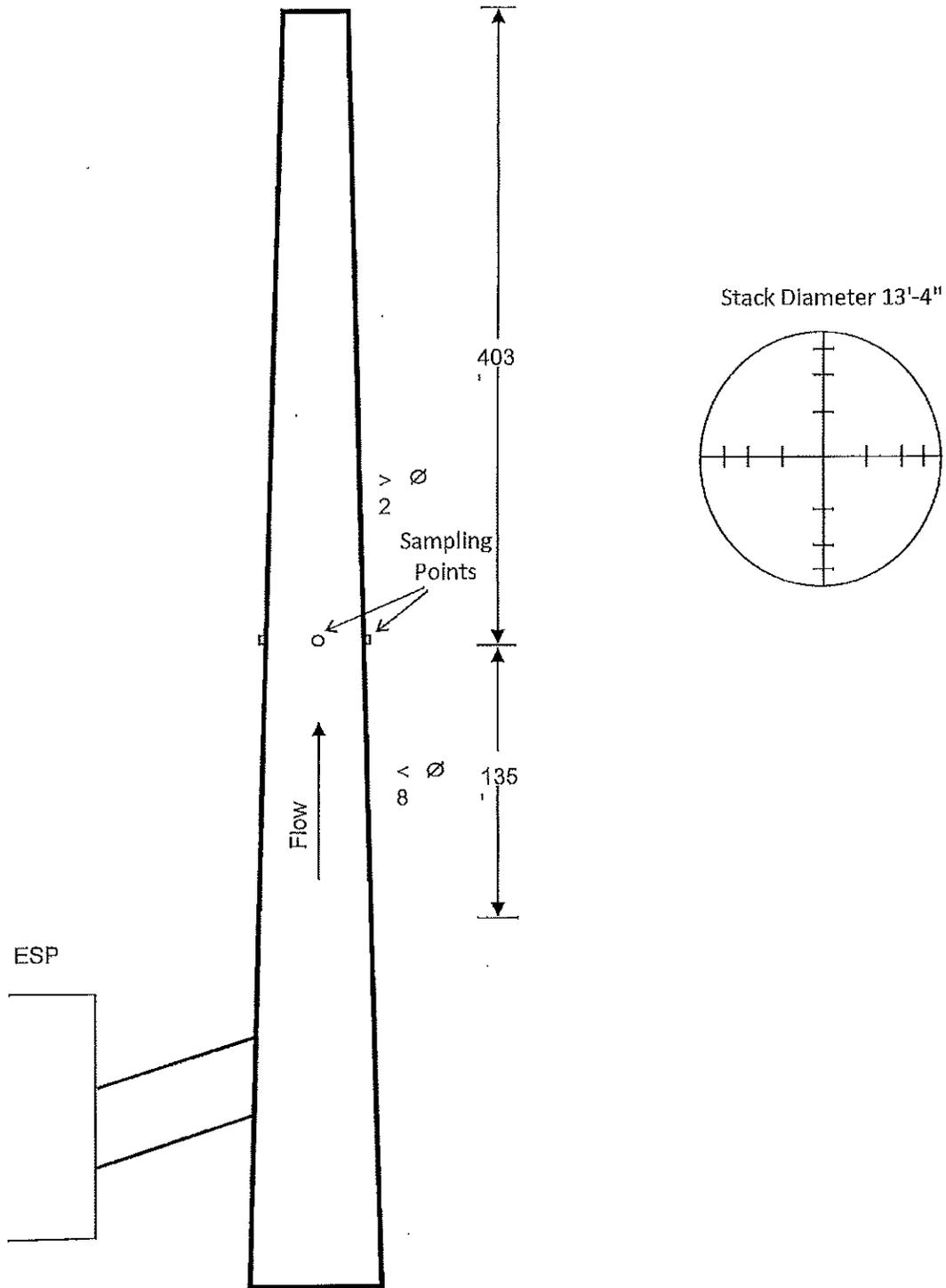
Figure 2 – USEPA Method 26A (Modified)
