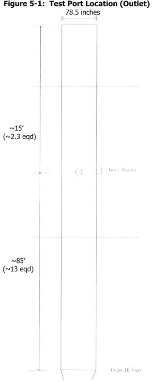
Figure 5-1: Test Port Location (Outlet)
