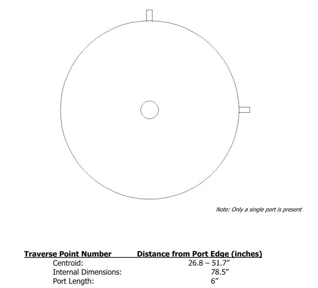
Figure 5-4: Sampling Point Locations (Outlet Ground Site)
