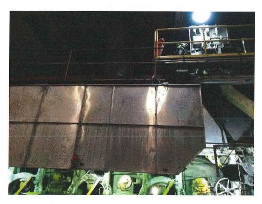
Image 3(Stack): Stack for first dryer of paper machine.
