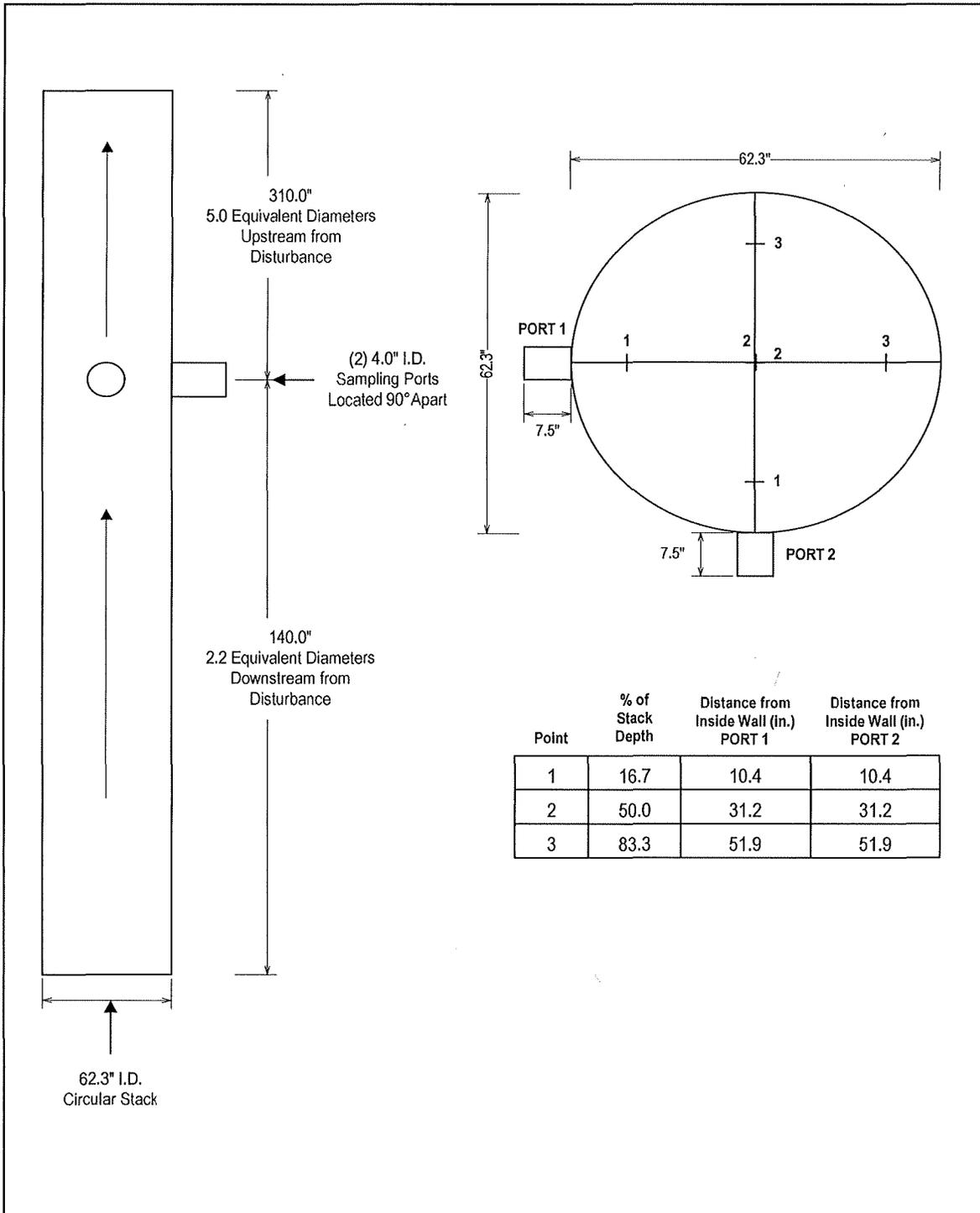
**EUBOILER#11 EXHAUST ISOKINETIC TRAVERSE POINT LOCATION DRAWING**
