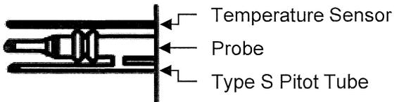
View of Probe End (from the bottom)
