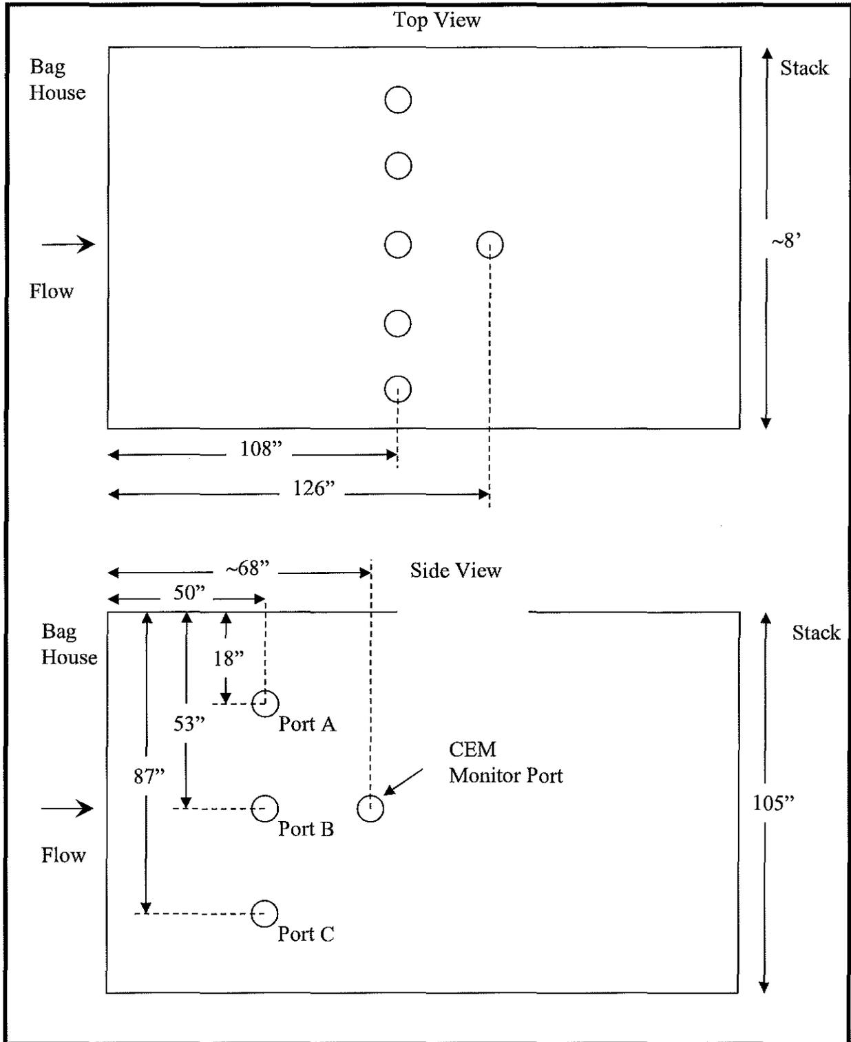
Figure 4-3. Lafarge Alpena Kilns 20 and 21 Breaching - Test Port Locations
