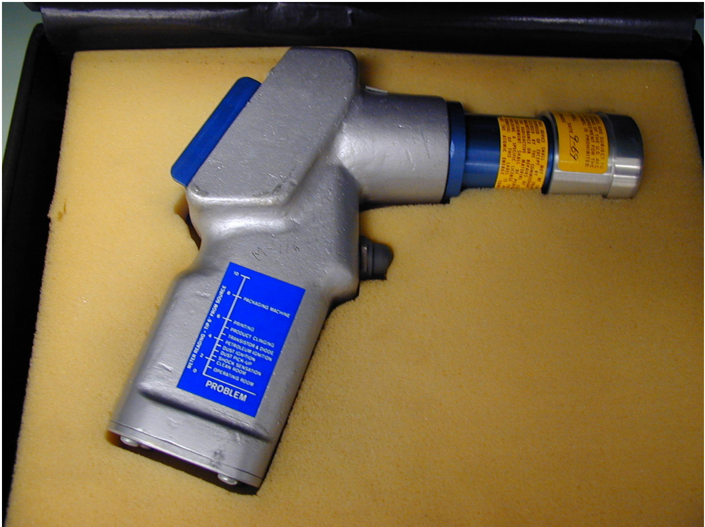
A static gun, containing a tritium (H-3) source.
