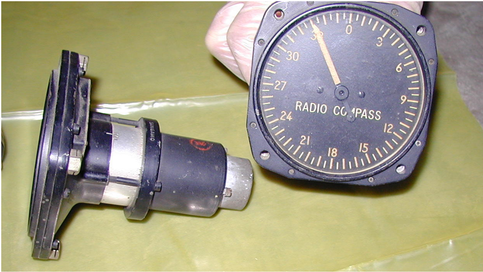
An aircraft compass with radium-painted hand and face. It no longer glows in the dark but is a strong gamma emitter.
