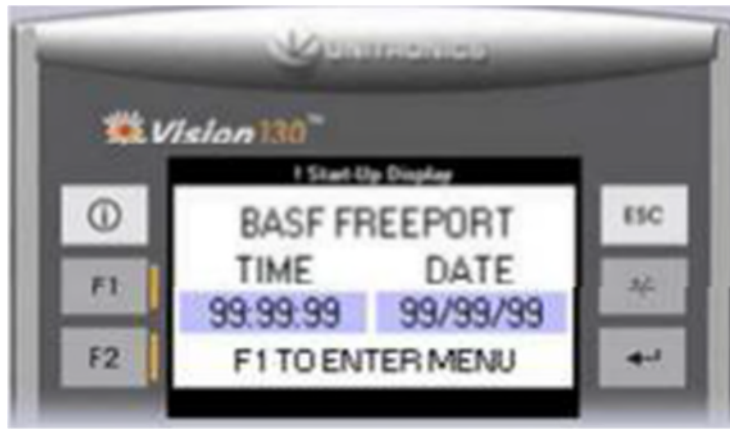
Figure 6. Operator Interface Controller Main Screen
