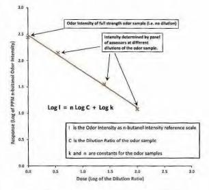
This Dose-Response, persistency, graph can be converted to a Power Law graph showing how the intensity changes with the odor concentration, represented in odor units. This conversion is completed by taking the recognition threshold of the odorous air sample, the full-strength odor concentration, into consideration.
