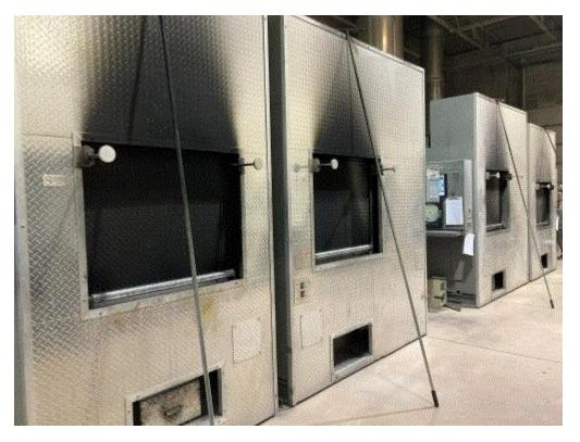
Image 2(IMG\_0135.JPGIMG\_0135) : View of soot deposits on the crematory doors. Image taken on February 10, 2020.
