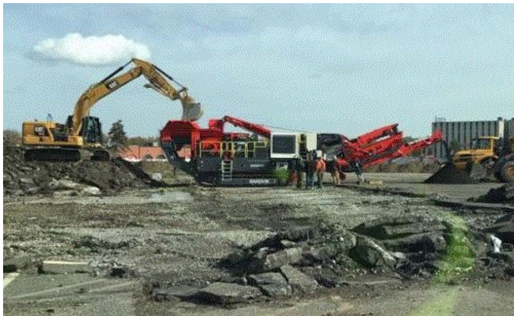
Image 1(IMG 7428 cropped) : Image from complainant of unpermitted nonmetallic mineral crushing activity. This image was received on 11/12/2021.
