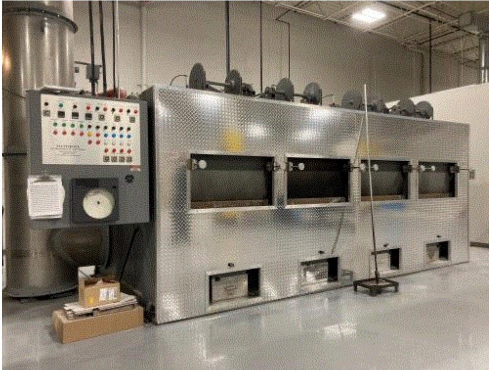
Image 4(IMG 0581) : Image of EUCREMATORY9. This is a 4-chamber animal cremation unit.
