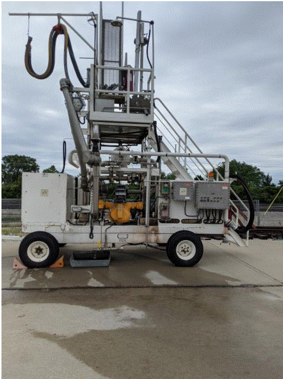
Image 1(Gantry Pump AV 400) : Portable Pump Unit for Fuel Transloading Operations
