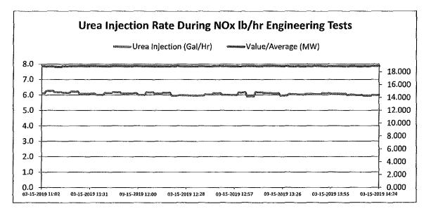
While UMERC had suspended the compliance testing, NOx pound/hour data was collected for engineering purposes during the remainder of the gaseous compliance testing on 3/15/2019. Final results of Run 1 and the engineering tests were obtained from Mostardi Platt several weeks after the compliance testing concluded. These results, which show compliance with applicable requiremetnts, are provided for informational purposes.
