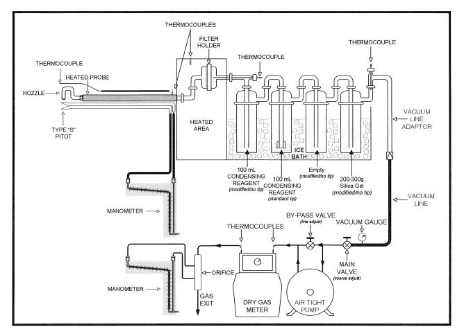
FIGURE 3-1 US EPA METHOD 5 SAMPLING TRAIN
