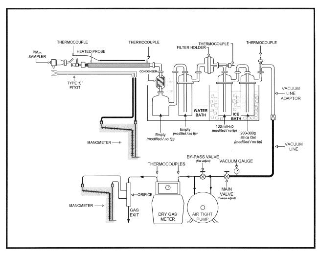
FIGURE 3-3 US EPA METHOD 201A (PM<sub>10</sub>/PM<sub>2.5</sub>)/202 SAMPLING TRAIN
