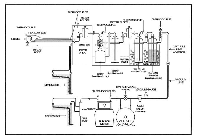
FIGURE 3-4 US EPA METHOD 5/202 SAMPLING TRAIN
