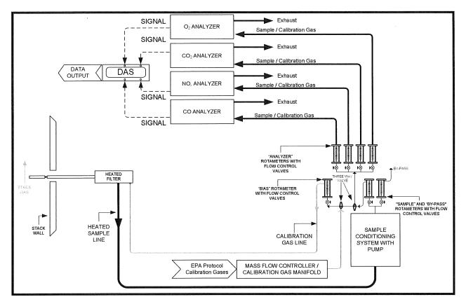
FIGURE 3-2 EPA METHODS 3A (O<sub>2</sub>/CO<sub>2</sub>), 7E, AND 10 SAMPLING TRAIN
