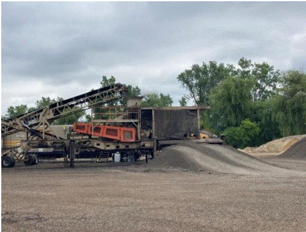
Image 1(KPI JCI 4250) : 500 tph primary jaw crusher
