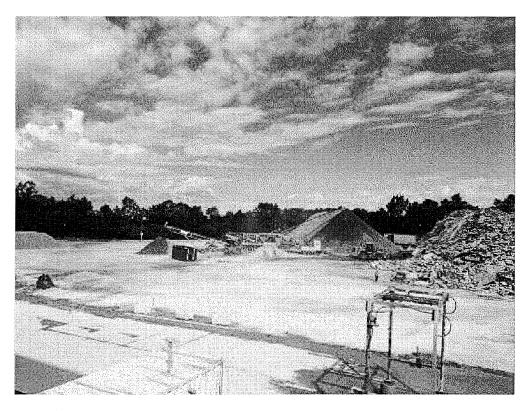
Image 2(Crushing facility) : Crusher on left, crushed pile in center, to be crushed pile on right. The truck wash station for Doan Companies can also be seen.
