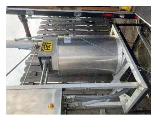
Image 1(Catalytic Oxidizer): Control device for remediation.
