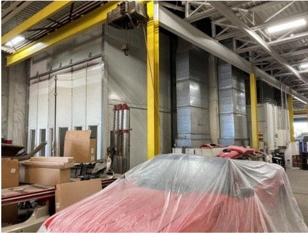
Image 4(IMG 0418) : EUBOOTH2 double-wide spray booth with a car in the foreground. This Emission Unit (EU) consists of two booths that are attached in the center. The large beige doors on the left are on the west side of the spray booth.
