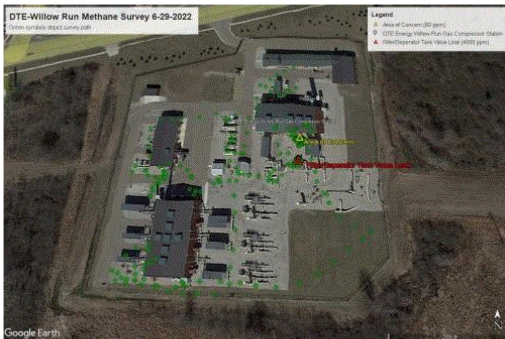
Image 1(Methane survey map) : Results of methane survey show one leak and one area of concern.
